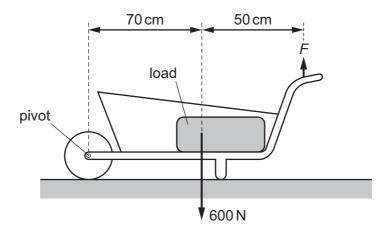
What is the size of force F needed just to lift the loaded wheelbarrow?
