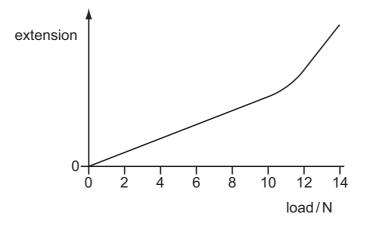
What is the total range of a balance with a linear scale using this spring?
