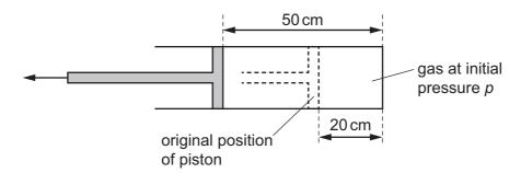
The piston is pulled out a distance of 30 cm, so that the length of the gas column is now 50 cm. The temperature of the gas does not change.
