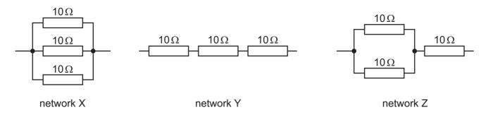
What is the order of resistance of the networks going from the smallest total resistance to the largest total resistance?
